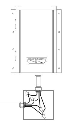
Connect the EmerGen Switch input wires to your permanent wiring as follows:
