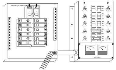
5. Identify the appropriate knockout to remove in the load center. 1-1/4" trade size is installed from the factory.
