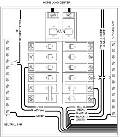
3. Repeat step 2 for each 120 volt circuit. See the following section for the installation of 240 volt circuits.
